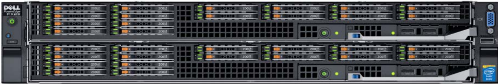
2 FC830 server blocks (each with 16 1.8" SSDs) in a fully loaded FX2 enclosure
